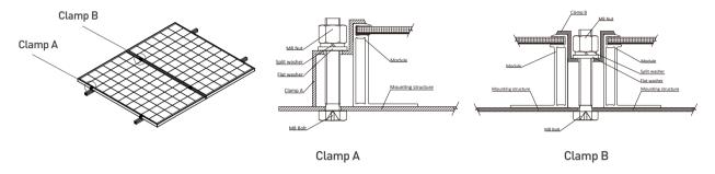
Figure 2 Clamp installation
