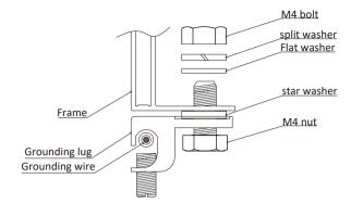
Figure 6 Grounding by cable
