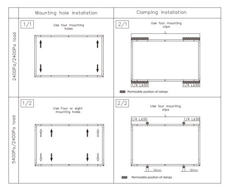
Figure3 Installation method
