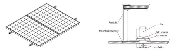
Figure 1 Mounting hole installation
